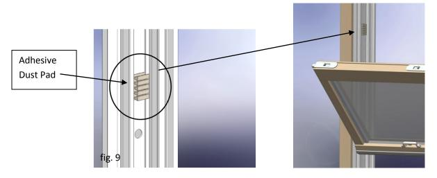
13. When the upper sash is in the fully raised position the adhesive pads should be located as shown in (fig. 10).
