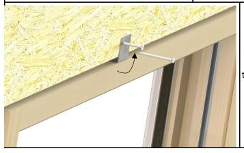
With window in the installed position, bend to 90 degrees and secure window to opening as shown with supplied screws.
